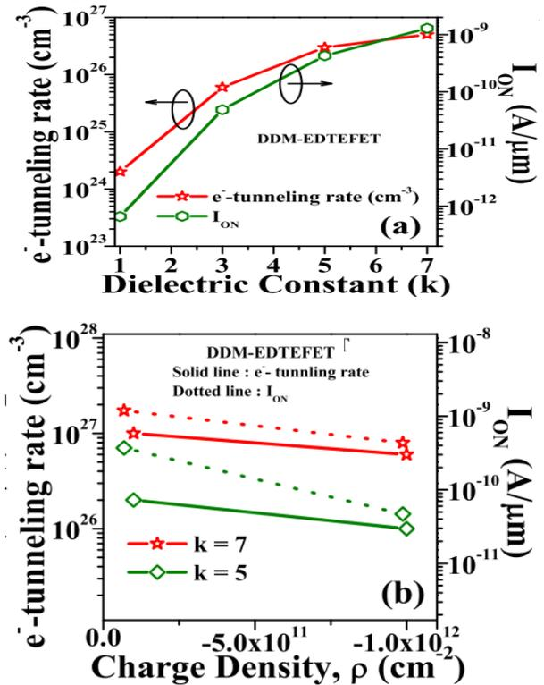
**Fig. 4.** Electron tunneling rate and ON-state current of DDM-EDTFET with different (a)  $k$  when  $\rho=0$  and (b)  $\rho$  when  $k=5$  and  $7$  under ON-state conditions ( $V_{DS} = 0.5V$  and  $V_{GS} = 1.2V$ ).
