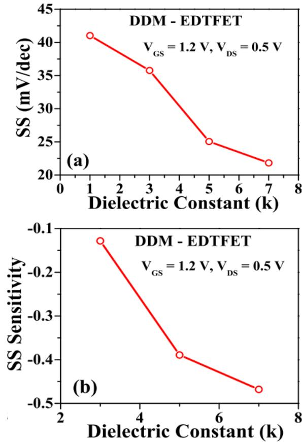
**Fig. 10.** (a) Subthreshold slope and (b) subthreshold slope sensitivity of the proposed device for  $\rho=0$  and dielectric range from  $k=1$  to  $7$  at  $V_{GS} = 1.2\text{V}$  and  $V_{DS} = 0.5\text{V}$ .
