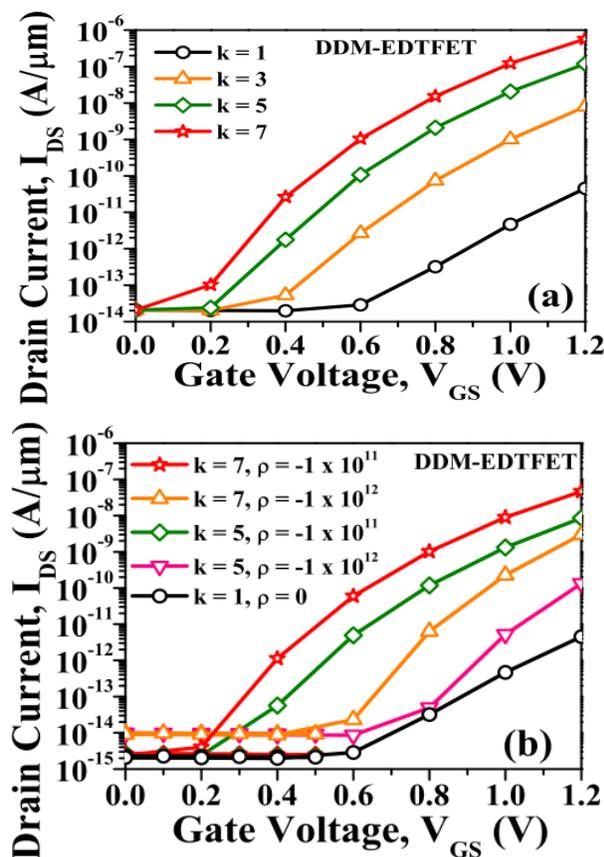
Fig. 6. Transfer characteristics of DDM-EDTFET with different (a)  $k$  when  $\rho = 0$  and (b)  $\rho$  when  $k = 5$  and  $7$  at  $V_{GS} = 1.2$  V and  $V_{DS} = 1$  V.
