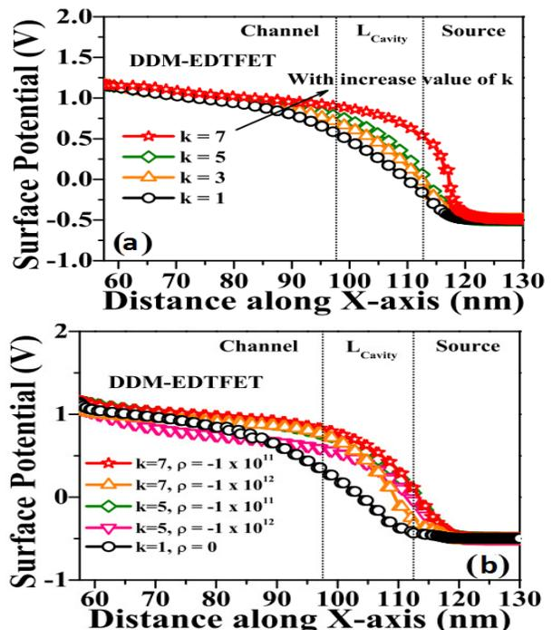
**Fig. 5.** Surface potential profile of DDM-EDTFET with different (a)  $k$  when  $\rho=0$  and (b)  $\rho$  when  $k=5$  and  $7$  under ON-state conditions ( $V_{DS} = 0.5V$  and  $V_{GS} = 1.2V$ ).
