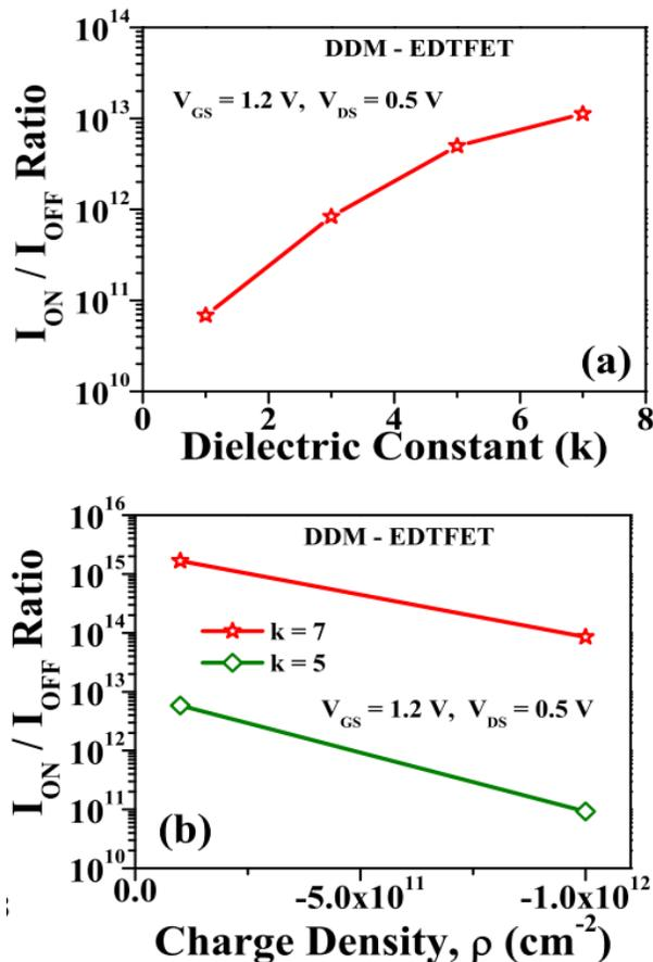
**Fig. 9.** Impact of charged biomolecules on (a)  $I_{ON}$  and (b)  $I_{ON}/I_{OFF}$  for a range of dielectric constant ( $k=5$ , and  $7$ ) for a DDM-EDTFET based biosensor at  $V_{GS} = 1.2V$  and  $V_{DS} = 0.5V$ .
