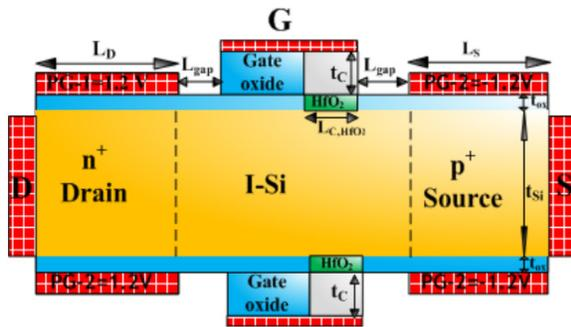
**Fig. 1.** Cross-sectional structural view of dual dielectrically modulated electrostatically doped tunnel-FET (DDM-EDTFET).
