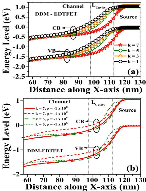
**Fig. 3.** Energy band diagrams of DDM-EDTFET along the X-axis with distinct values of (a)  $k$  when  $\rho = 0$  and (b)  $\rho$  when  $k = 5$  and  $7$  under ON-state conditions ( $V_{DS} = 0.5V$  and  $V_{GS} = 1.2V$ )
