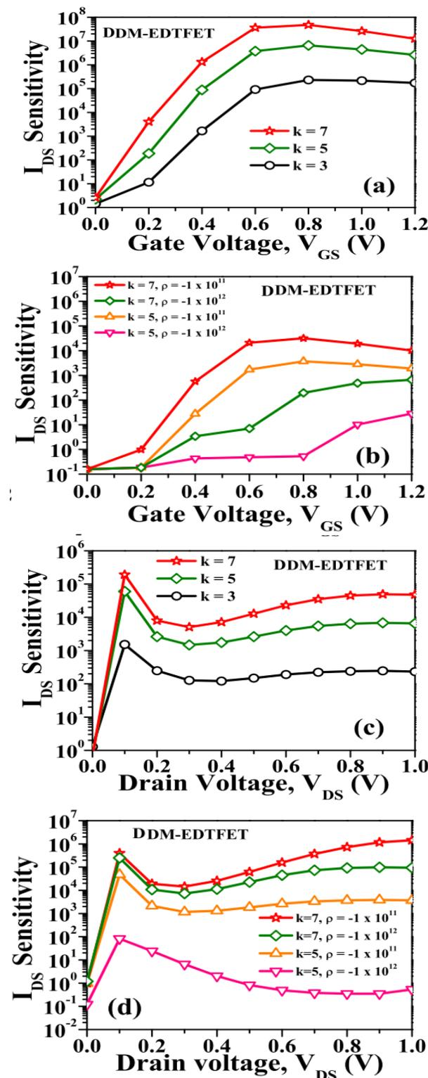
**Fig. 8.** Drain current sensitivity of DDM-EDTFET with different (a)  $k$  but  $\rho=0$  and (b)  $\rho$  but  $k=5$  and  $7$ ; with  $V_{GS}$  variation at a fixed  $V_{DS} = 0.5V$ . Drain current sensitivity of DDM-EDTFET with different (a)  $k$  but  $\rho=0$  and (b)  $\rho$  but  $k=5$  and  $7$  with  $V_{DS}$  variation at a fixed  $V_{GS} = 1.2V$ .
