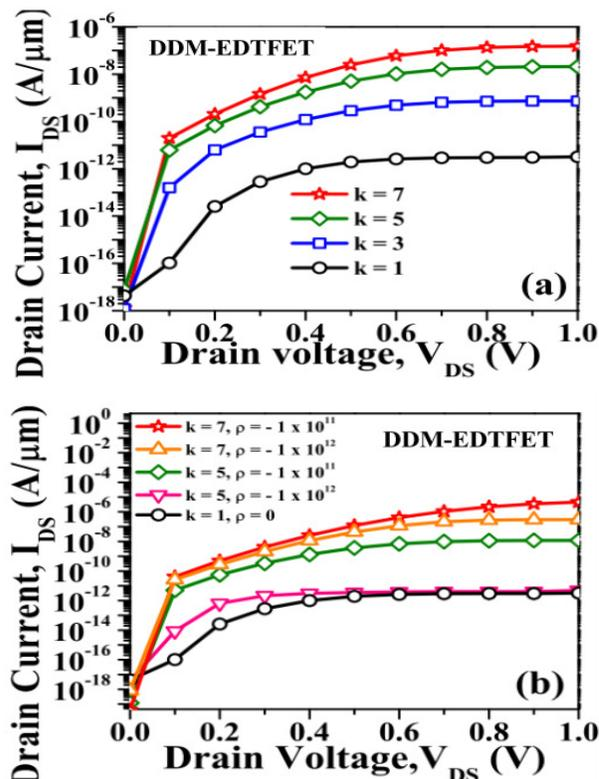
Fig. 7. Output characteristics of DDM-EDTFET with different (a)  $k$  when  $\rho = 0$  and (b)  $\rho$  when  $k = 5$  and  $7$  at  $V_{GS} = 0.5$  V and  $V_{DS} = 1$  V.
