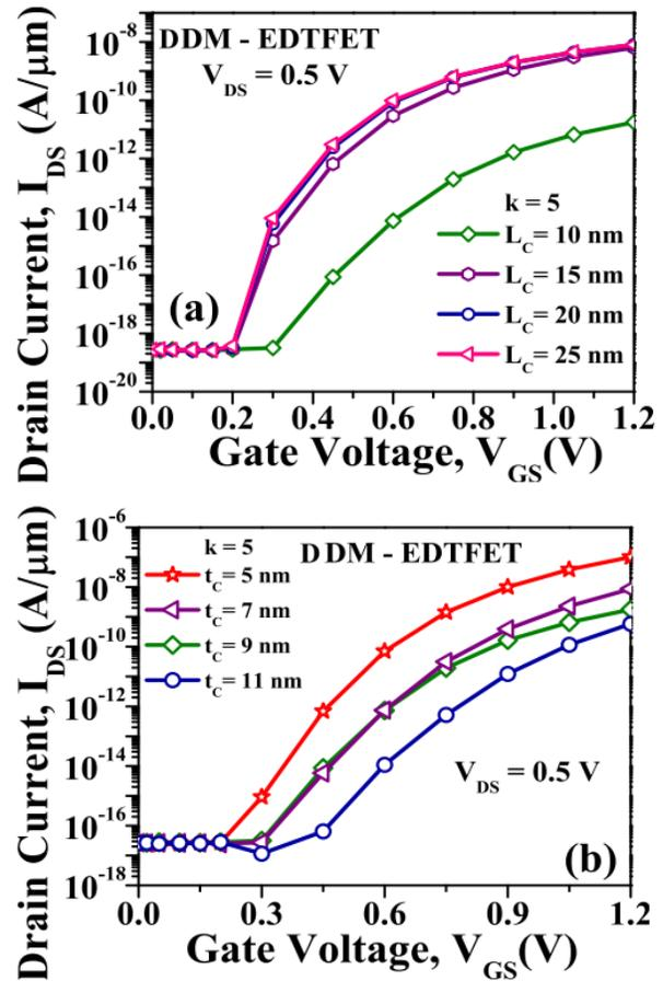
**Fig. 11.** Effect of variation in (a) the length of cavity ( $L_C$ ) and (b) the thickness of cavity ( $t_c$ ) on the transfer characteristics of DDM-EDTFET at  $V_{GS} = 1.2\text{V}$  and  $V_{DS} = 0.5\text{V}$ .
