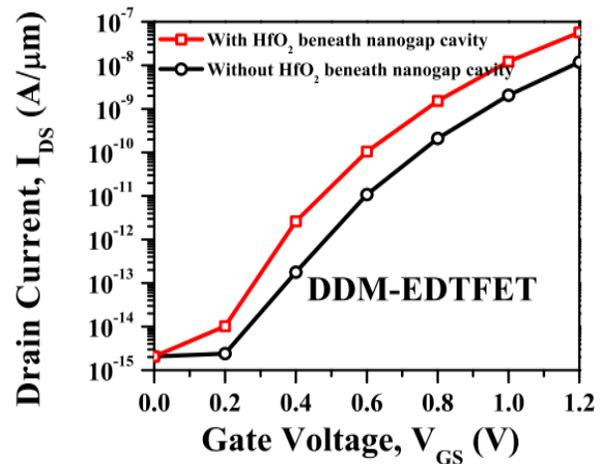
**Fig. 2.** Transfer characteristics of DDM-EDTFET with and without high-k material,  $\text{HfO}_2$  as an insulator in the nanogap cavity filled with biomolecules with dielectric constant,  $k=5$  at  $V_{\text{DS}} = 1.0 \text{ V}$  and  $V_{\text{GS}} = 1.2 \text{ V}$ .
