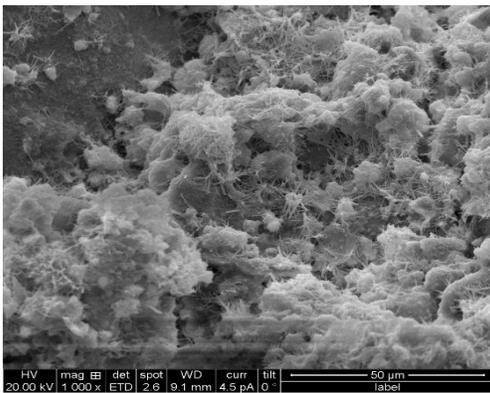
Fig. 8. SEM image at 30% replacement of GGBS.
