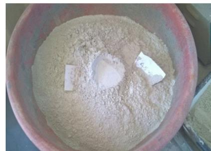
Fig. 1. Ground granulated blast furnace slag (GGBS).
