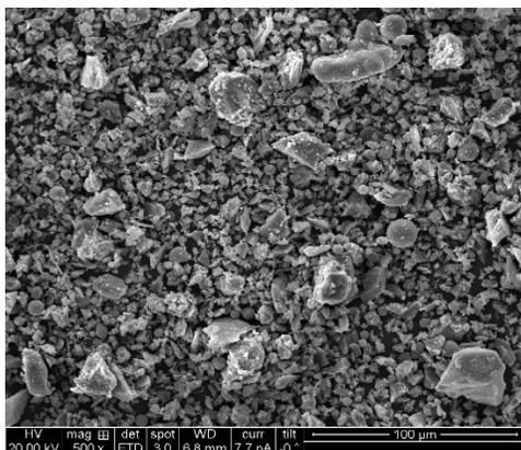
**Fig. 2.** SEM image for cement.
