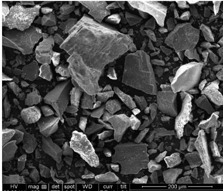
**Fig. 4.** Shows the SEM image for M-sand.
