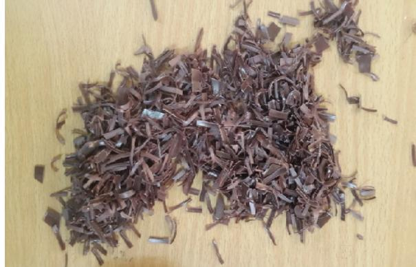
**Fig. 1.** Photograph of PPF used in this study.
