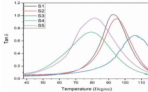
**Fig. 6.** Tan  $\delta$  v/s temperature curve for neat epoxy and sisal composites.
