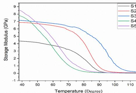
**Fig. 4.** Storage Modulus vs. Temperature curves for Prepared Specimens.
