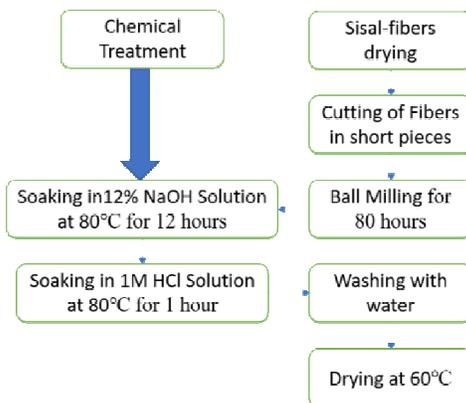
**Fig. 1.** Flowchart of alkali treatment of sisal fibre.
