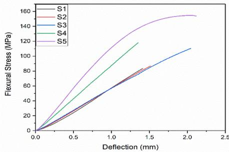
**Fig. 3.** Flexural stress v/s deflection curve of neat epoxy and sisal composites.
