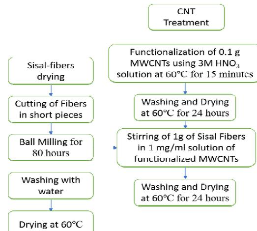
**Fig. 2.** Flowchart for the CNT treatment of Sisal-fibres.
