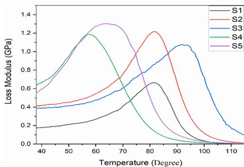
**Fig. 5.** Loss modulus v/s temperature curves for neat epoxy and sisal composites.
