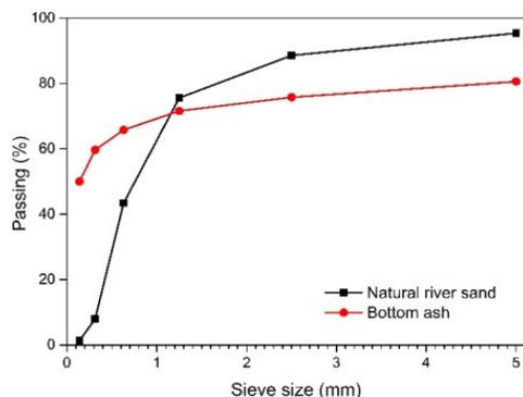
Fig. 1. Gradation curves of natural river sand and CBA.
