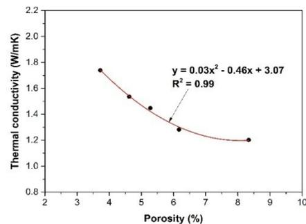
Fig. 10. The relationship between TC and porosity of concretes.
