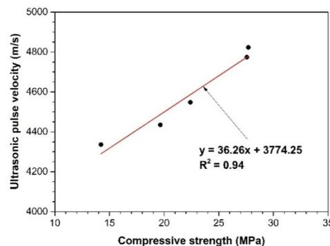
Fig. 5. Relationship between UPV and compressive strength of concretes.
