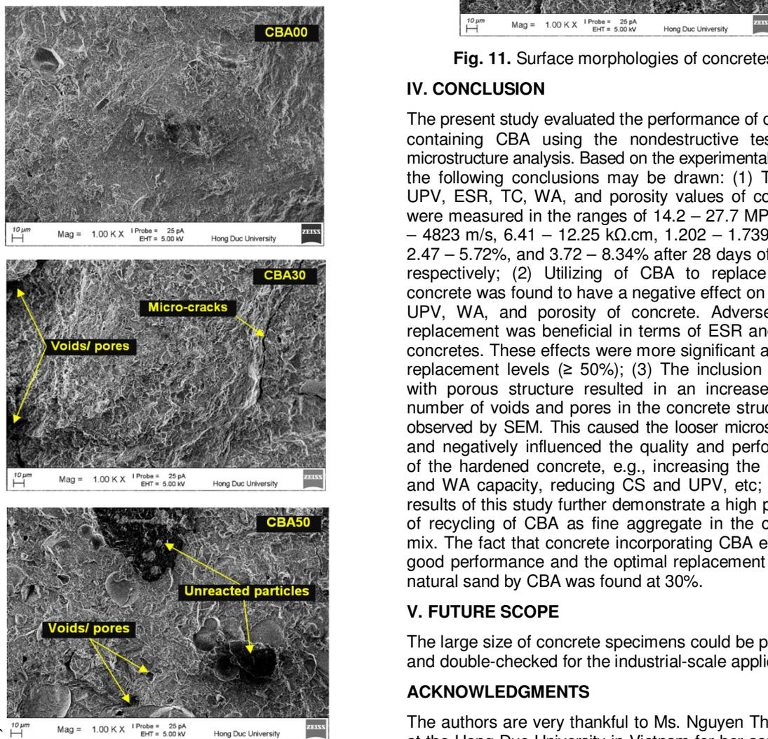
Fig. 11. Surface morphologies of concretes.
