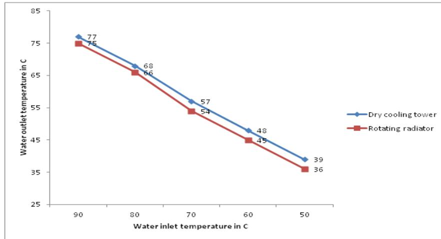
Fig. 11. Comparison of water outlet temperature.
