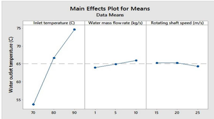
Fig. 10. The graphical response of water outlet temperature with varying the input parameters.
