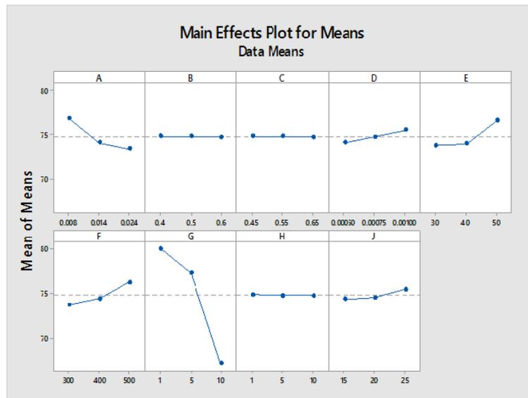
**Fig. 8.** Mean effect of parameters to water outlet temperature.
