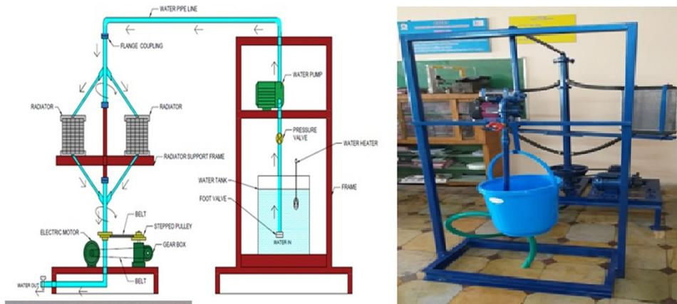
**Fig. 3.** Schematic and photograph of the experimental setup.
