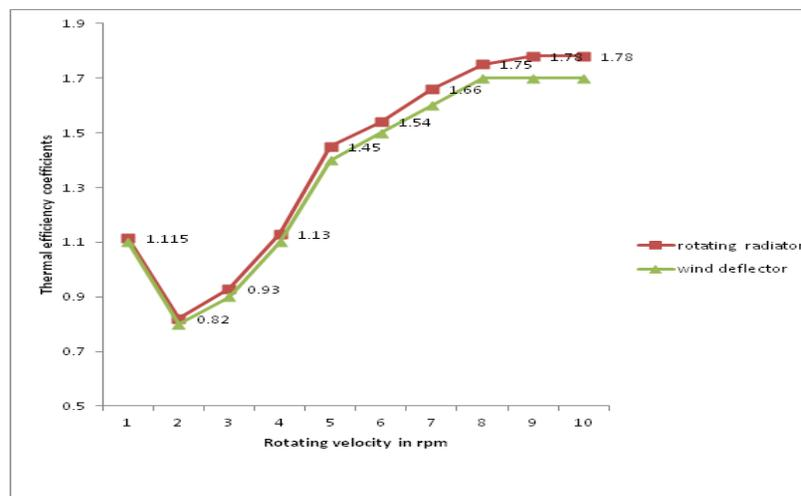
Fig. 12. Comparison of thermal efficiency of rotating radiator with wind deflectors [6].
