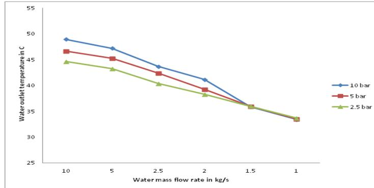
**Fig. 7.** Graph representing water outlet temperature for varying pressure and mass flow rate.
