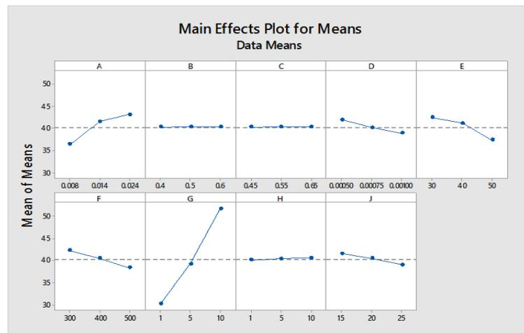
**Fig. 9.** Mean effect of parameters to Air outlet temperature.
