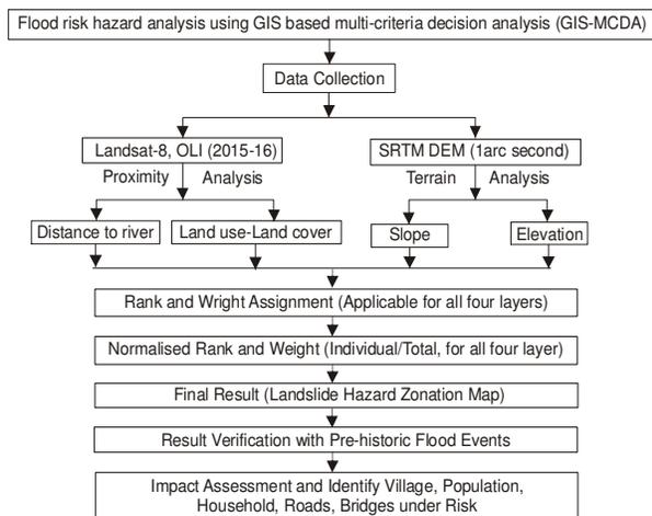
**Fig. 2.** Flow diagram of methodology used for GIS-MCDA based flood hazard zonation mapping.
