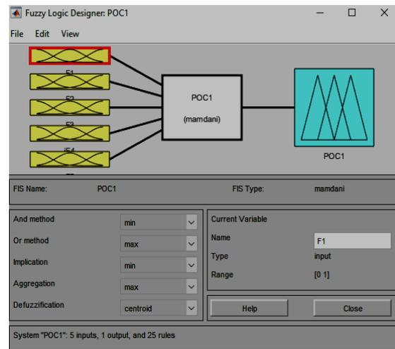
**Fig. 26. Defining Input and output variables.**
