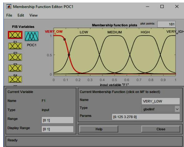
**Fig. 27. Defining membership of Input and output variables.**
