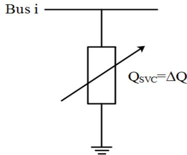
**Fig. 1.** The injections of ΔQ as size of SVC at Bus i.
