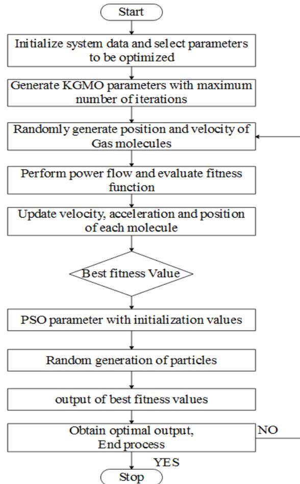
Fig. 5. Flowchart of Hybrid KGMO-PSO algorithm.
