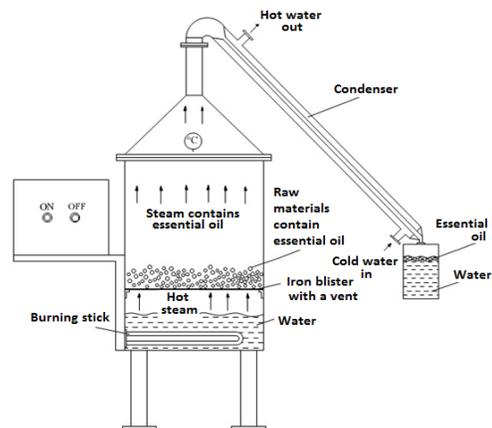
**Fig. 1.** Diagram of steam distillation system.
