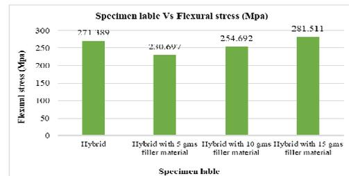
Fig. 11. Graph between the name of the specimen and the flexural stress of the specimen.
