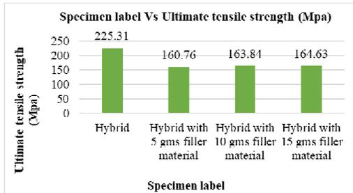
Fig. 6. Graph between the name of the specimen and the tensile strength of the specimen.
