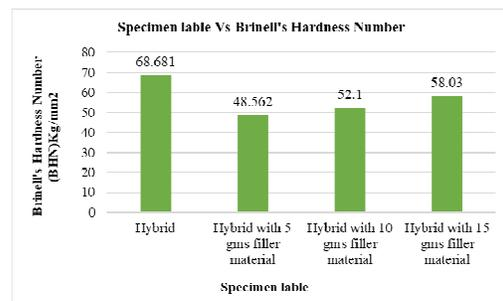
Fig. 13. Graph between the name of the specimen and hardness number of the specimen.
