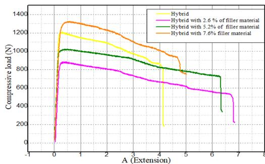
Fig. 9. Graph for compressive extension against compressive load for all composite specimens.
