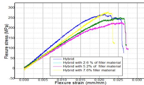
Fig. 12. Graph for flexural strain against flexural stress for all composite specimens.
