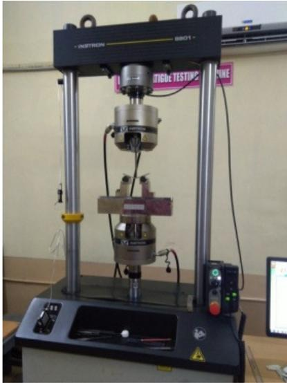
Fig. 2. INSTRON 8801 testing machine.
