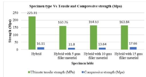
Fig. 10. Graph between the name of the specimen and the relative tensile strengths and compression.
