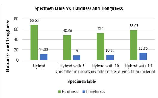
Fig. 15. Graph between the name of the specimen and their relative hardness and toughness.
