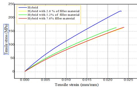
Fig. 7. Stress-strain curve for all composite specimens.
