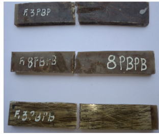
Fig. 5. Samples after flexural testing.
