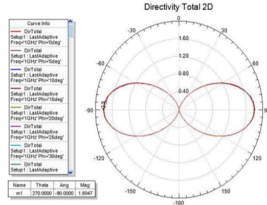
**Fig. 17.** Directivity characteristics of modified design using HFSS tool.
