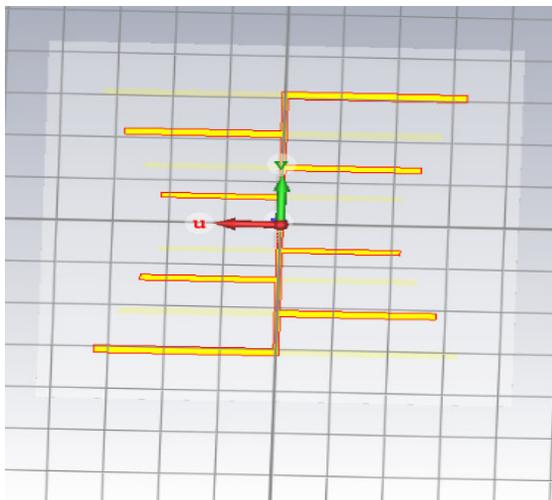
**Fig. 6.** Back view of Log Periodic Dipole Array Antenna (using CST).
