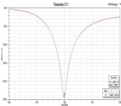
**Fig. 15.**  $S_{11}$  of LPDA with modifications using HFSS tool.
