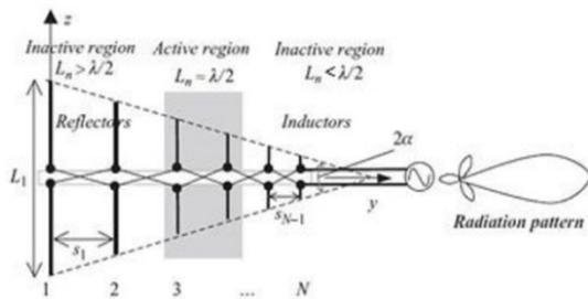
**Fig. 1.** Log Periodic Dipole Array Antenna
