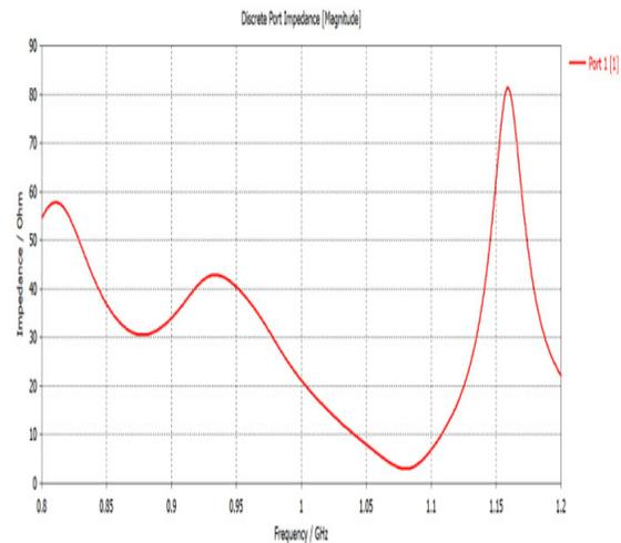
**Fig. 8.** The measured impedance of the antenna before modifying the antenna design using CST.
