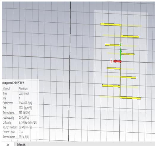
**Fig. 5.** Front view of modified Log Periodic Dipole Array Antenna (using CST)
