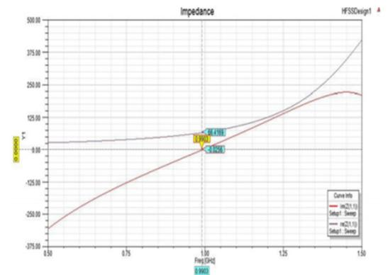
**Fig. 16.** Impedance characteristics of modified design using HFSS tool.
