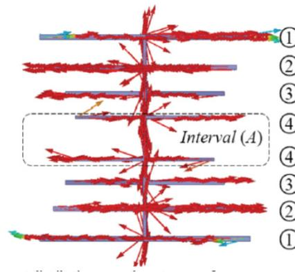
**Fig. 3.** Current flow across the antenna before modifying the antenna design parameters.
