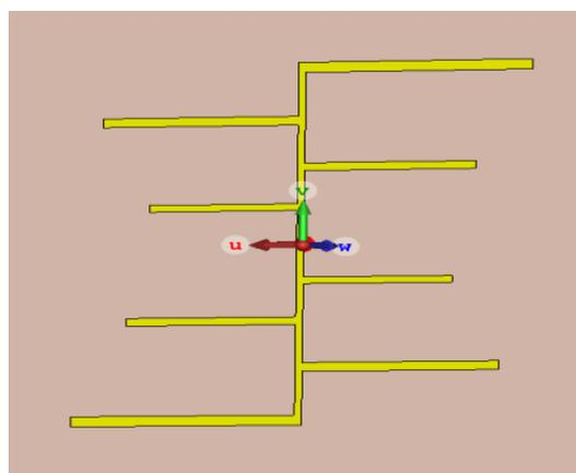
**Fig. 4. Structural Design of modified Log Periodic Dipole Array Antenna.**
