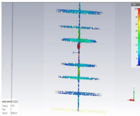
**Fig. 10.** The current distribution of the typical LPD antenna, without modification.
