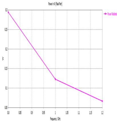
**Fig. 9.** The radiated power of the typical structure of DLPA, before implementing the modification, using CST.
