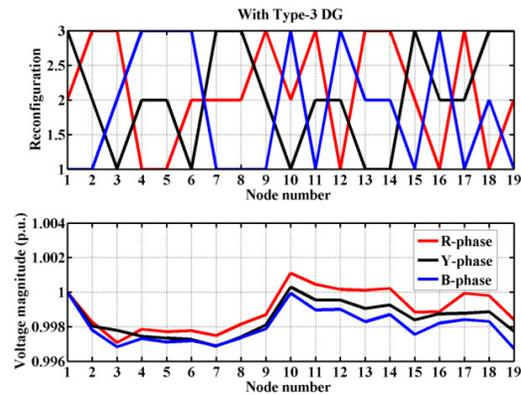
**Fig. 10.** Variation of node voltage and phase reconfigurations with Type-3 DG for URDS-19 node system.
