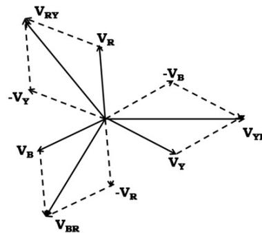
Fig. 5. Phasor simplification to calculate phase voltage.
