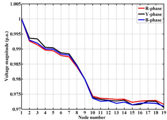
Fig. 6. Variation of voltage magnitude for URDS-19 node system.
