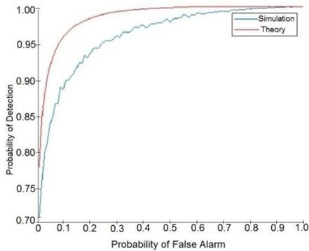
**Fig. 3.** ROC plots for the energy detector at SNR 10dB.
