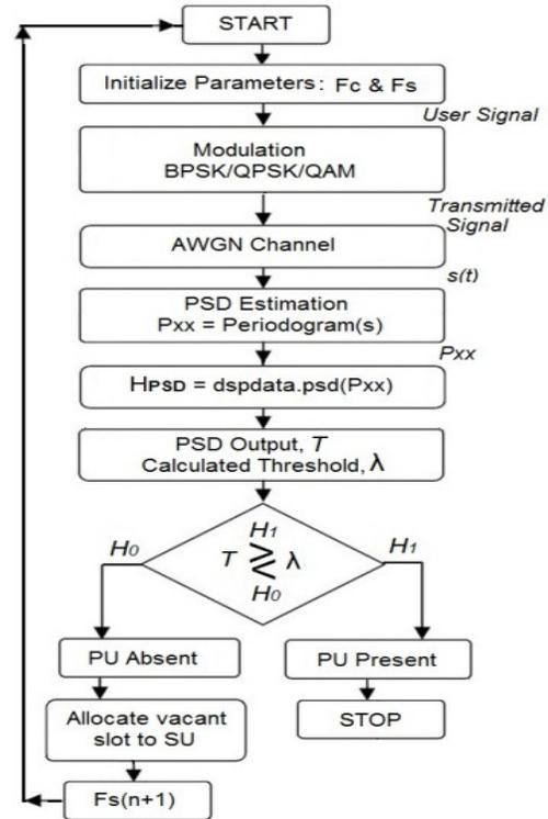
Fig. 1. Flow chart for PSD based energy detection.
