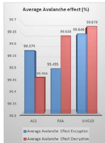
Fig. 3. Average Avalanche effect (%) of existing methods and SHIELD model.
