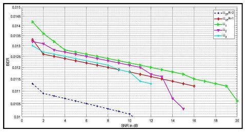
Fig. 6. BER performance of Modified μ law companding technique on SCM-OFDM system with different companding levels U<sub>1</sub>,U<sub>2</sub> and U<sub>3</sub>.Table IV: Comparison of PAPR Reduction techniques for SCM-OFDM system.
