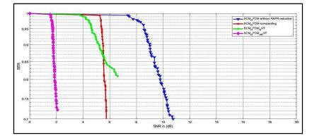
Fig. 8. BER performance of different PAPR reduction technique on SCM-OFDM system.
