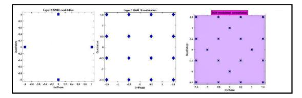
Fig. 3. Simulation result of Superposition Coded Modulation of two signals QPSK and 16 QAM modulated signal.
