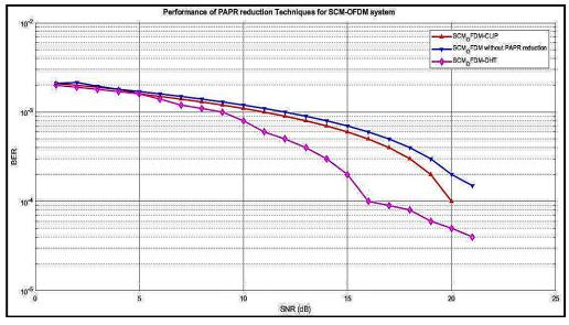
Fig. 4. BER performance of Clipping and DHT PAPR reduction techniques in SCM-OFDM system.
