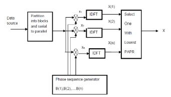
Fig. 2. Block diagram of Selective Mapping.
