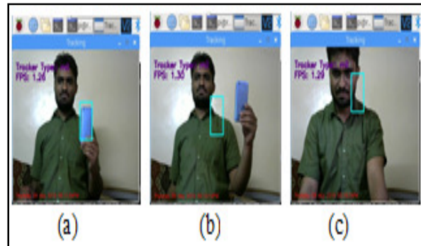
Fig. 8. Tracking results for cellular phone in frames (a), (b) and (c) with MIL Tracker.
