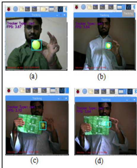
Fig. 5. Tracking results of ball in given frames (a), (b), (c) and (d) with CSRT tracker at great accuracy.
