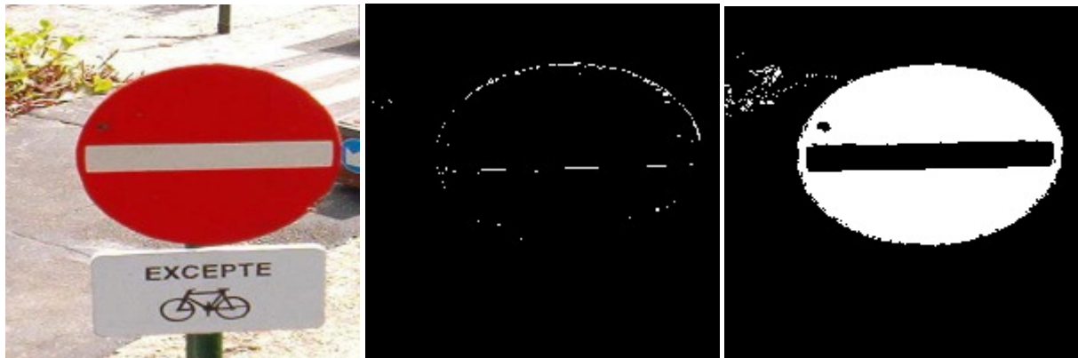
(a) Original image (b) For the threshold [\min, 255] (c) For the threshold [\min - 40, 255]
