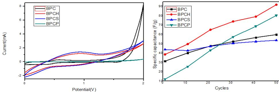
**Fig. 3** (a) CV curves of BPC, BPCH, BPCS and BPCP a scan rate of 30 mVs<sup>-1</sup>, (b) Cycle stability of BPC, BPCH, BPCS and BPCP.
