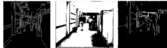
Fig. 3 (a) Multiple texture extraction (b) Adaptive threshold object. (c) Segmented image.
