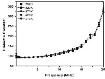
Fig. 2. Variation of dielectric constant of  $MgFe_2O_4$  ferrite with frequency at different temperatures.
