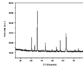
Fig. 1. XRD patterns of  $MgFe_2O_4$  sample sintered at 1373K.
