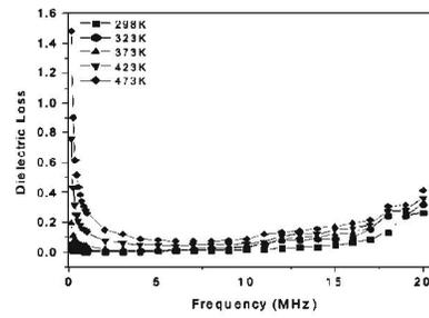
Fig. 4 Variation of dielectric loss of  $MgFe_2O_4$  ferrite with frequency measured at different temperatures.
