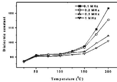
Fig. 3. Variation of dielectric constant of  $MgFe_2O_4$  ferrite with temperature at different frequencies.
