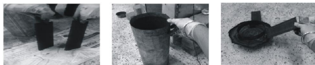
Fig 2. Soot collected from Electrode (2a), Detachable Chimney (2b) and Canopy (2c) of the electrical precipitator unit
