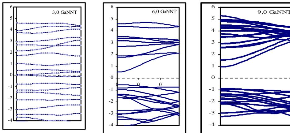
Fig. 1. Band structure of (3,0), (6,0) and (9,0) of GaNNTs.
