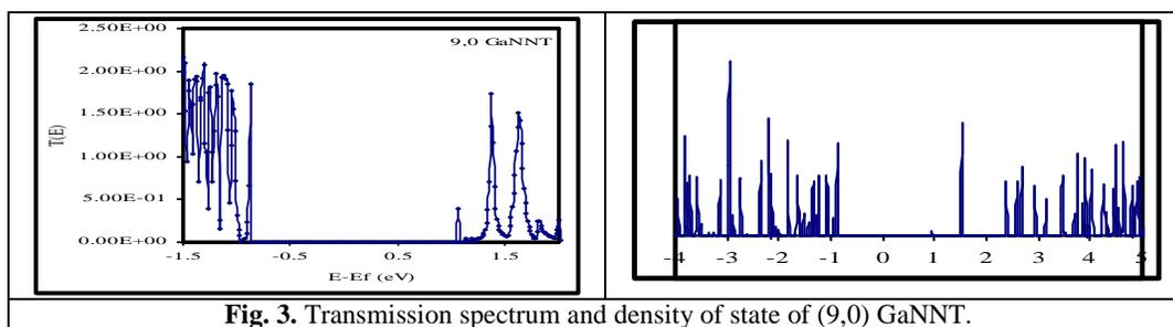
Fig. 3. Transmission spectrum and density of state of (9,0) GaNNT.
