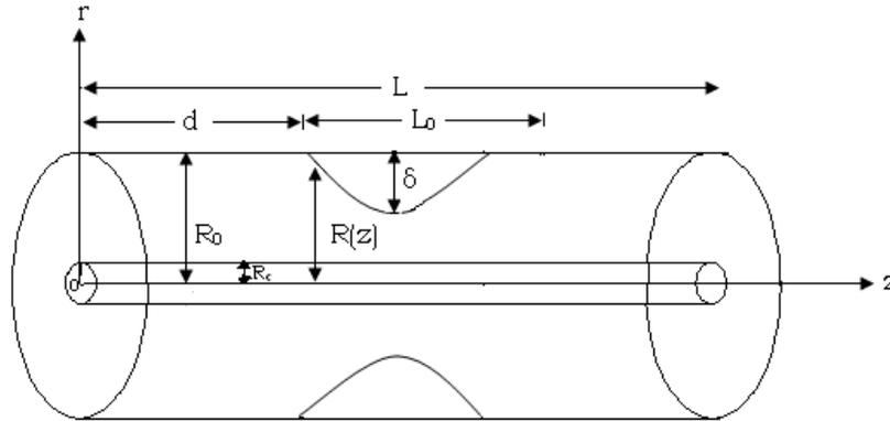
**Fig. 1.** Flow geometry of stenosis in a catheterized artery.
