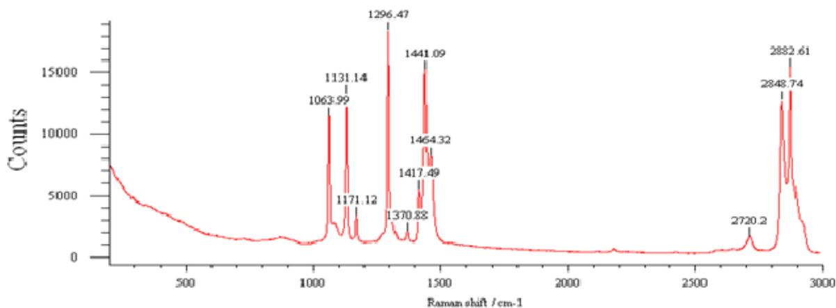
**Fig.1.** Polyethylene (Control).
