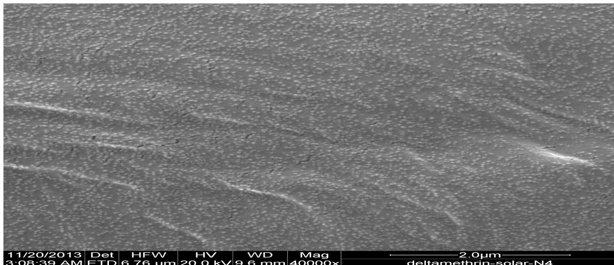
**Fig. 1(c)** SEM of Solar Exposed DM Filament.
