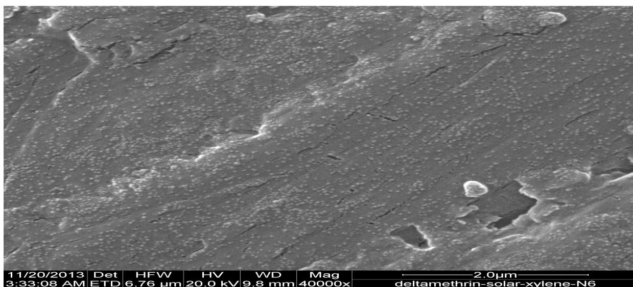
**Fig. 1(d)** SEM of Solar Exposed xylene treated DM Filament.
