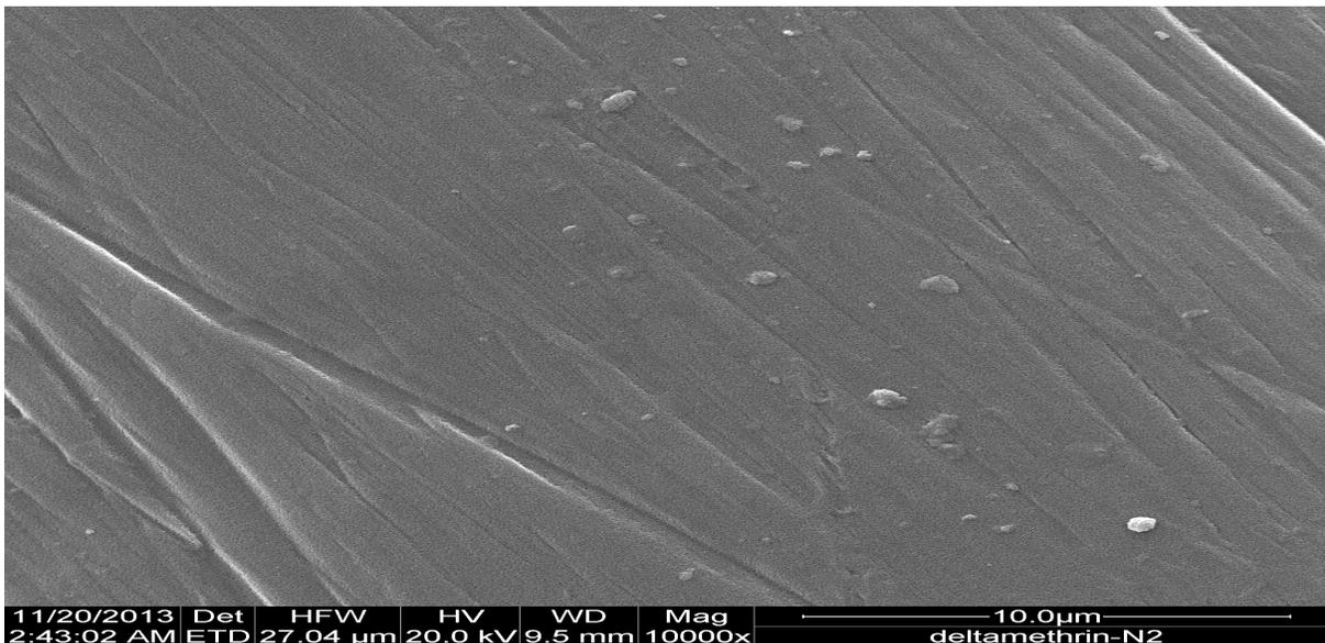
Fig. 1(a) SEM of DM doped unexposed polyethylene filament.
