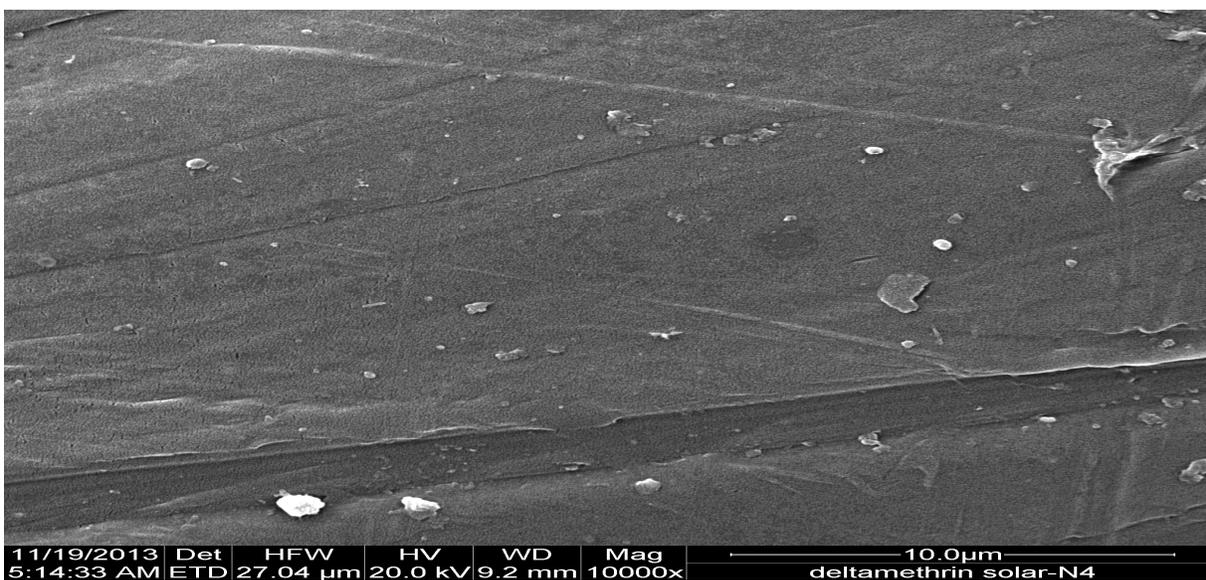
Fig. 1(b) SEM of Solar Exposed DM Filament.
