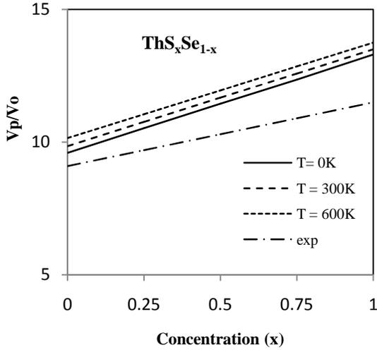
**Fig. 5.** Variation of  $V_p/V_o$  with concentration ( $x$ ).
