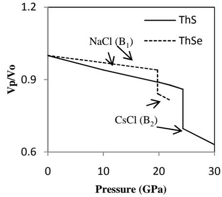
**Fig. 3.** Variation of  $V_p/V_o$  with pressure for ThS and ThSe.
