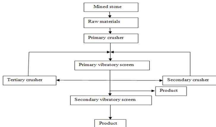
Fig. 1. Stone crushing process flow
