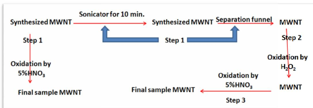
Fig. 1. Schematic of purification process for synthesized MWNTs.
