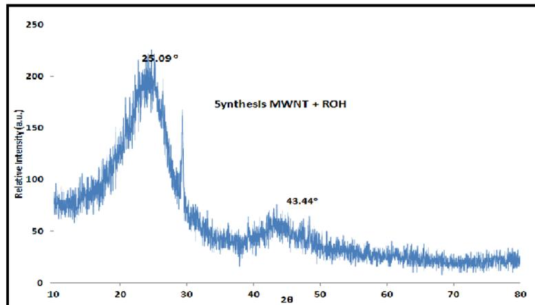
Fig. 5. XRD patterns of synthesized MWNTs after treatment with ethanol in exist of ultra-sonic water bath.
