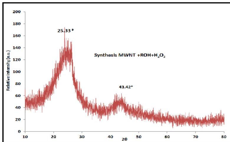
Fig. 6. XRD patterns of synthesized MWNTs after treatment with ethanol in exist of ultra-sonic water bath than with H<sub>2</sub>O<sub>2</sub>.
