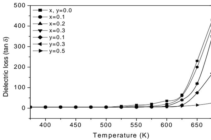
Fig.7 Variation of dielectric loss with temperature for  $Mg_{0.9}Mn_{0.1}In_xFe_{2-x}O_4$  and  $Mg_{0.9}Mn_{0.1}Al_yFe_{2-y}O_4$  ferrites at 1 kHz
