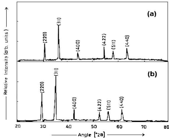
Fig.1. X-ray patterns of (a) Mg<sub>0.9</sub>Mn<sub>0.1</sub>In<sub>0.1</sub>Fe<sub>1.9</sub>O<sub>4</sub> and (b) Mg<sub>0.9</sub>Mn<sub>0.1</sub>Al<sub>0.1</sub>Fe<sub>1.9</sub>O<sub>4</sub> ferrite powders sintered at 1200<sup>o</sup>C
