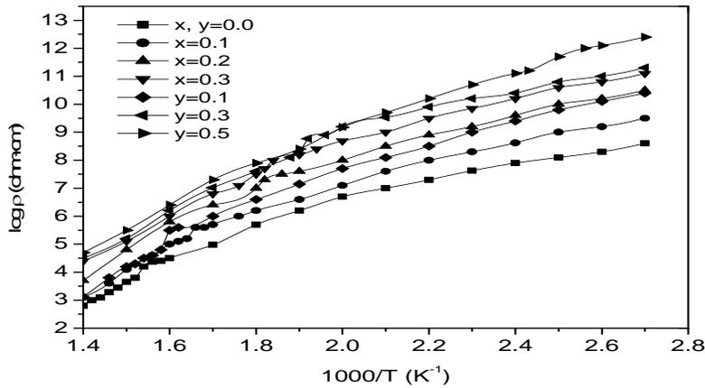
Fig.3. Variation of resistivity with temperature for  $Mg_{0.9}Mn_{0.1}In_xFe_{2-x}O_4$  and  $Mg_{0.9}Mn_{0.1}Al_yFe_{2-y}O_4$  ferrites
