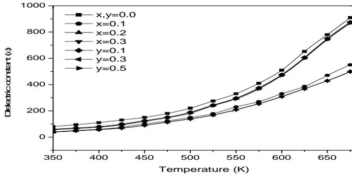
Fig.5 Variation of dielectric constant with temperature for  $Mg_{0.9}Mn_{0.1}In_xFe_{2-x}O_4$  and  $Mg_{0.9}Mn_{0.1}Al_yFe_{2-y}O_4$  ferrites at 1kHz.
