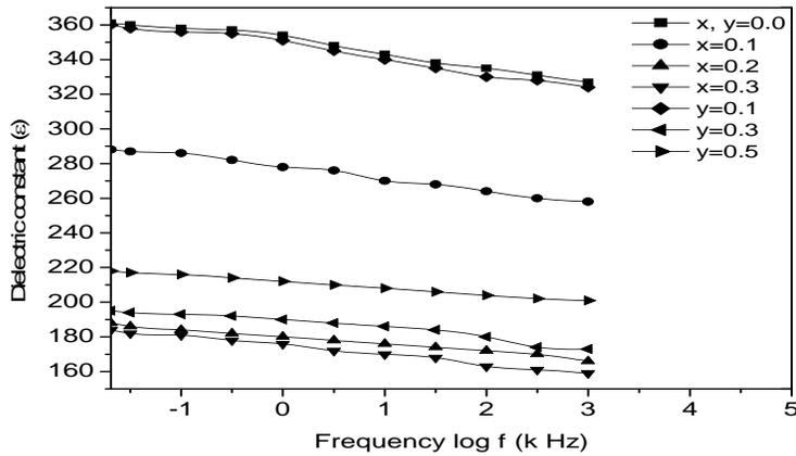
Fig.4 Variation of dielectric constant with frequency for  $Mg_{0.9}Mn_{0.1}In_xFe_{2-x}O_4$  and  $Mg_{0.9}Mn_{0.1}Al_yFe_{2-y}O_4$  ferrites
