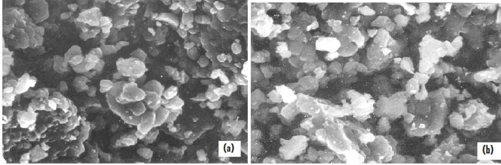
Fig.2. Scanning electron micrographs (SEM) of fractured surfaces for (a)  $Mg_{0.9}Mn_{0.1}In_{0.1}Fe_{1.9}O_4$  and (b)  $Mg_{0.9}Mn_{0.1}Al_{0.1}Fe_{1.9}O_4$  ferrites sintered at  $1200^{\circ}C$
