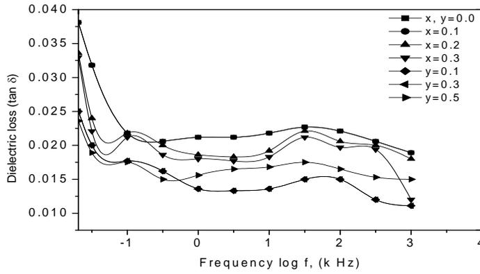
Fig.6 Variation of dielectric loss with frequency for  $Mg_{0.9}Mn_{0.1}In_xFe_{2-x}O_4$  and  $Mg_{0.9}Mn_{0.1}Al_yFe_{2-y}O_4$  ferrites
