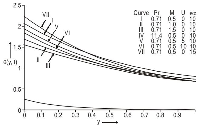
Fig.3. Temperature profiles versus  $y$  for  $Sc = 0.22$ ,  $Gr = 10$ ,  $Gc = 10$ ,  $\omega = 30$  and  $\omega t = \pi/4$ .
