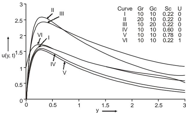
Fig.1. Velocity profiles versus  $y$  for  $Pr = 0.71$ ,  $M = 10$ ,  $\varepsilon\alpha = 10$  and  $\omega t = \pi/4$ .
