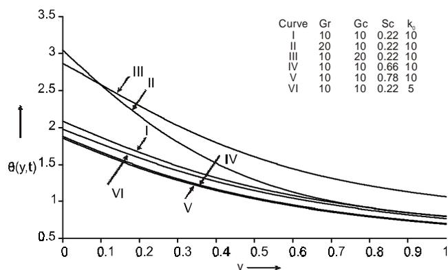
Fig.4. Temperature profiles versus  $y$  for  $Pr = 0.71$ ,  $M = 0.5$ ,  $Ec = 0.001$  and  $\omega t = \pi/4$ .
