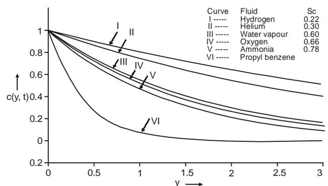
Fig.5. Concentration profiles for  $\omega = 30$ ,  $\varepsilon = 0.005$  and  $\omega t = \pi/4$ .
