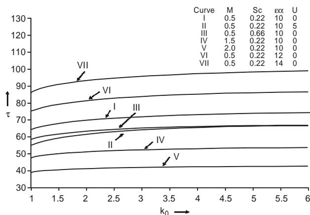
Fig.6. Skin-friction coefficient versus  $k_0$  for  $Pr = 11.4$ ,  $Gr = 5$ ,  $Gc = 3$ ,  $\omega = 10$  and  $\omega t = \pi/4$ .
