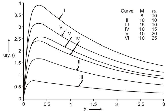
Fig.2. Velocity profiles versus  $y$  for  $Pr = 0.71$ ,  $Sc = 0.22$ ,  $Gr = 10$ ,  $Gc = 10$ ,  $\omega = 30$  and  $\omega t = \pi/4$ .
