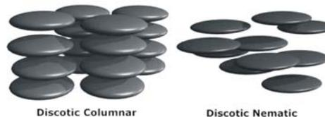
Fig. 8. The structure of nematic and columnar phases of disc like molecules.
