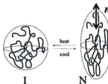
Fig. 10. Change of average molecular shape from spherical to spheroidal.
