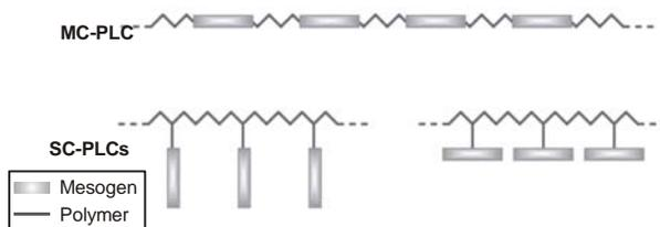
**Fig. 9.** Structure for MC-PLC and SC-PLC.
