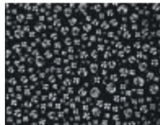
**Plate : 2.** Texture of Polymer Dispersed Liquid Crystal.
