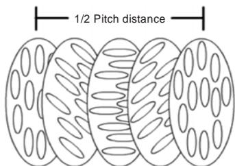
(b) The rotation of directors in a continuous helical pattern about the layer normal.
