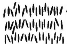
(a) Molecular arrangement in a SmA phase. The long axes of the molecules in each layer, on an average, are  $\perp$  to the layer containing the molecules.
